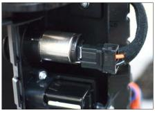
=> If the cup holder has a solid bottom you have to drill a hole (diameter of 18 mm) in order to install the USB connector cable
